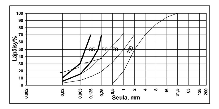
Sand in the 35 Mpa -area might be susceptible for frost heave and must be used in dry conditions
